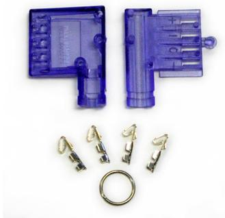
Simply solder or crimp wires from a four conductor cable to each of the four clips, and line them up in the right hand piece with the spring ends protruding through the slots to the outside of the connector, keeping track of which wire is going to which spring clip.
