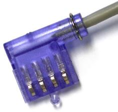
Now, you can solder or crimp the wires from the cable to the appropriate pins on your serial connector (DB-9, DB-25, or Mini DIN-8). Refer to the "Connector Pinouts and Signals" diagrams on the reverse side as this page, as well as the following electrical construction guidelines to wire your connector appropriately.
